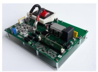
Singular modules can be exchanged during operation, facilitating a simple maintenance. Defect or old battery cells can be substituted with more modern cells. ©Fraunhofer ISE
